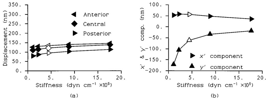
FIG. 5. Variation of in-plane annular-ligament stiffness. Effects on (a) out-of-plane component of displacement and (b)  $x'$  and  $y'$  components of translation. The input is a pure tone of 100 dB SPL.
