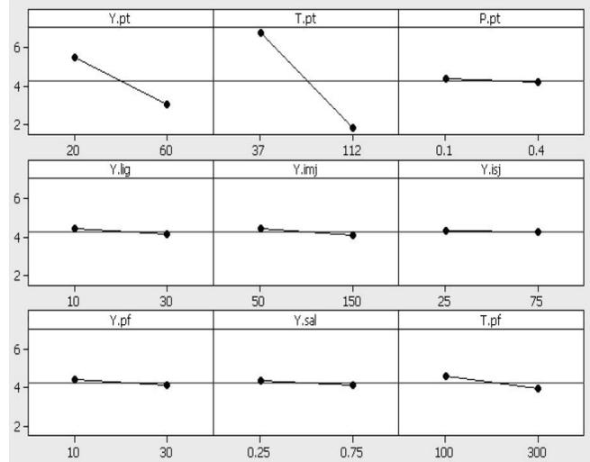
Figure 1: Parameters' main effects on TM volume displacement
