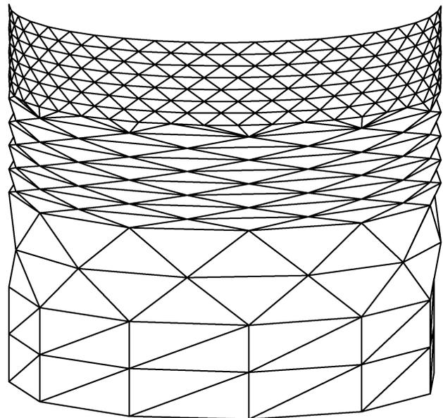
Figure 1. The front surface of a cylinder, triangulated in four layers. For the bottom two layers,  $n = 2$  and  $k = 11$ . For the third layer  $n$  is increased to 8 while  $k$  is still 11. For the fourth layer  $n$  is kept at 8 while  $k$  is increased to 40.
