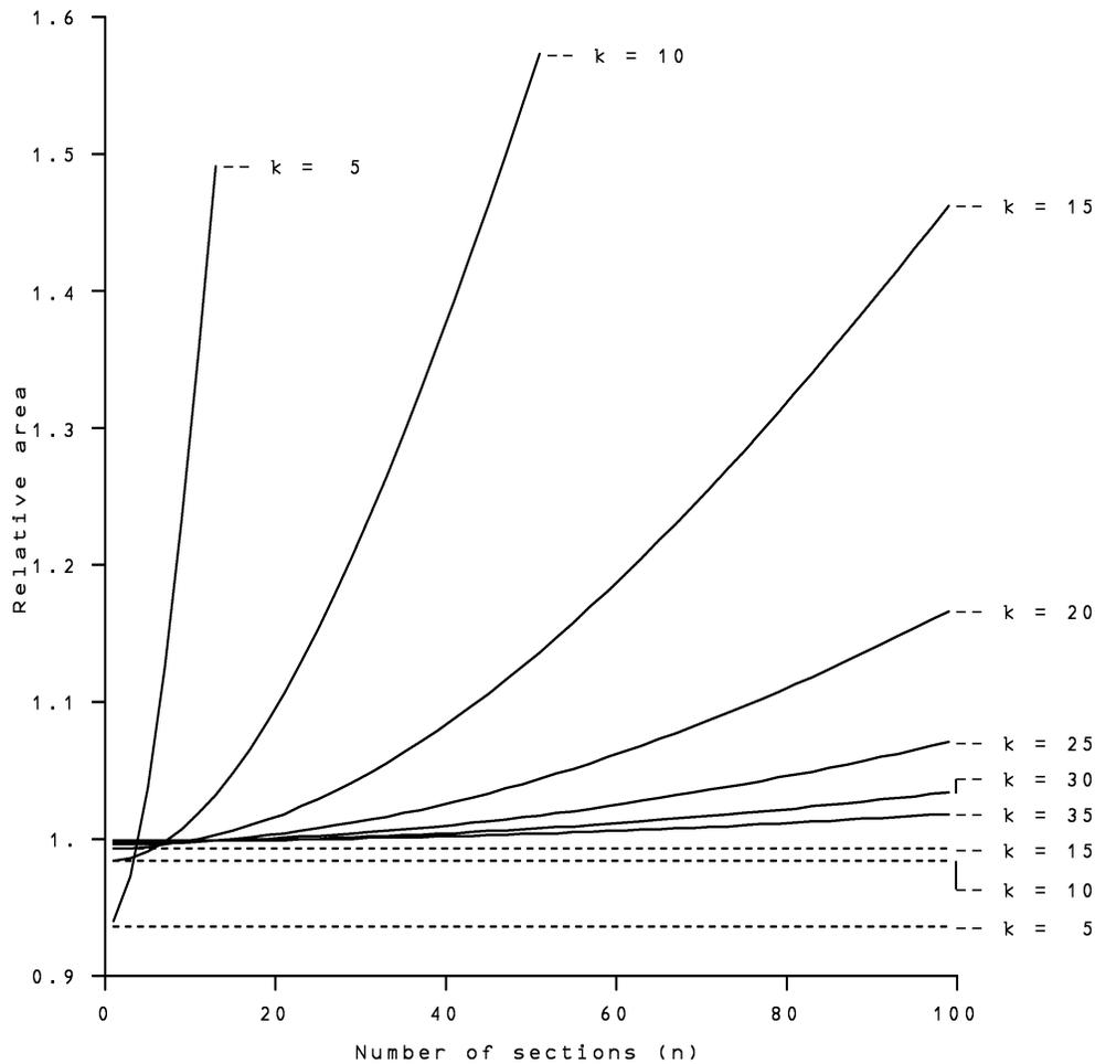
Figure 2. Relative area (estimated area divided by true area) as a function of  $n$ , for various values of  $k$ , for a triangulation with staggered nodes (solid lines) and for one with nodes that are not staggered (broken lines).
