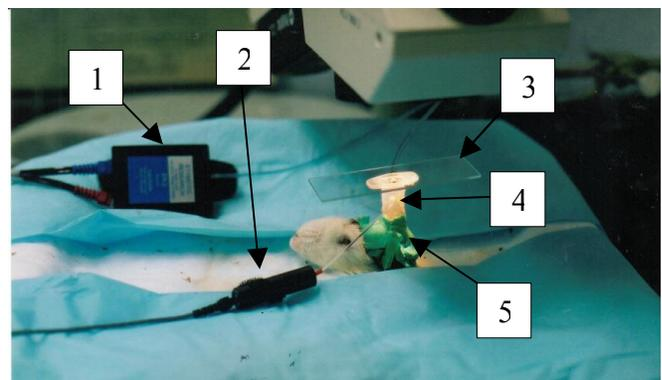
**Figure 3** Photograph of experimental setup. 1 = ER-2 Tubeophone™, 2 = ER-7C probe microphone system, 3 = glass cover slip, 4 = sound chamber, 5 = Plasticine™
