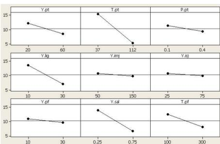
Figure 7. Parameters' main effects on footplate displacement
