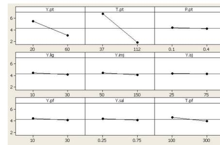
Figure 2. Parameters' main effects on TM volume displacement
